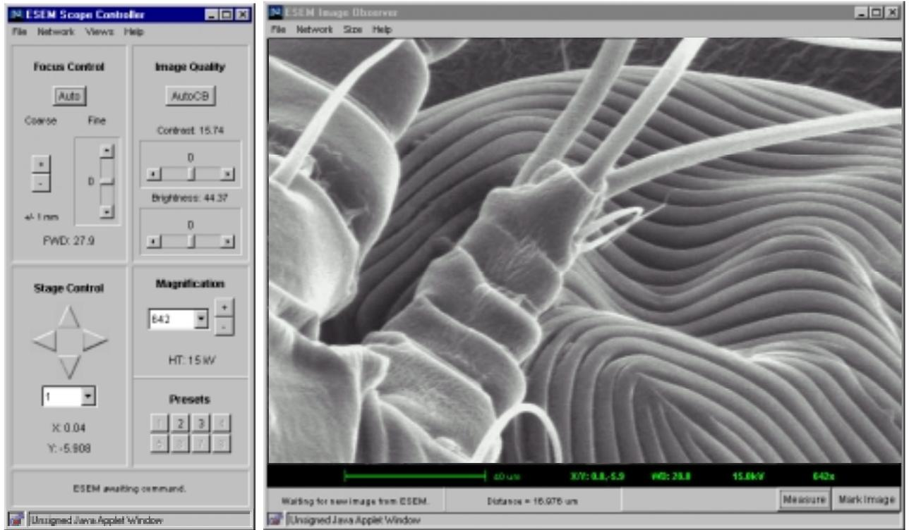
**Figure 1:** The microscope controller (left) and image observer (right) used for the Bugscope Project. These Java Applets are launched by a standard web browser from a classroom computer and used to interface the students to the instrument via the Internet. Access to the controller requires a password but the observer may be launched by any group interested in watching the progress of the experiment.
