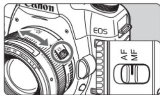
**1 Set the lens focus mode switch to <MF>.**
