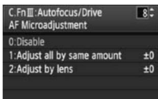
You can make fine adjustments for the AF's point of focus. It can be adjusted in  $\pm 20$  steps (-: Forward / +: Backward).
