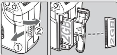
**Open the slot cover and insert a card.** (p.29)
