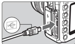
**3** Connect the camera to the printer.
